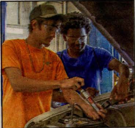
Austin Kortzendorf and Mayki Jones checking radiator pressure.
